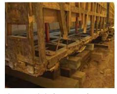
The two end platforms were far beyond saving and were scrapped to prepare for leveling the car.
