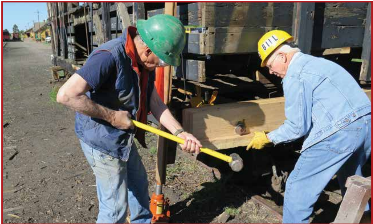
Sometimes a small hammer just doesn't quite do the job! Dave Ferro and Bill Lock install (persuade?) a new end sill onto Sheep Car 5600 during Special Session SS2 in May. To learn more about "Special Sessions," see Pages 16 and 17. There is another view of Car 5600 on Page 17 as well.
