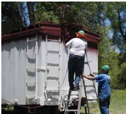
Stripped and primed in 2022, the repaint of #163 begins by painting the roof and ends of the car Boxcar Red in June 2023.
