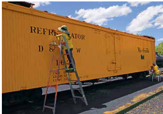
Gayle Mecca stencils in the reporting marks on the car (top) and touches up the bold text on the car. Photos by Mike Mee
