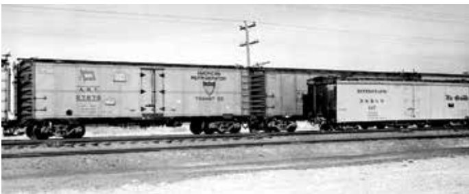
Like S Gauge vs. HO Gauge, there is a noticeable difference between narrow gauge 40-foot Long Reefer 167 and the 40-foot A.R.T. Car 27678.
