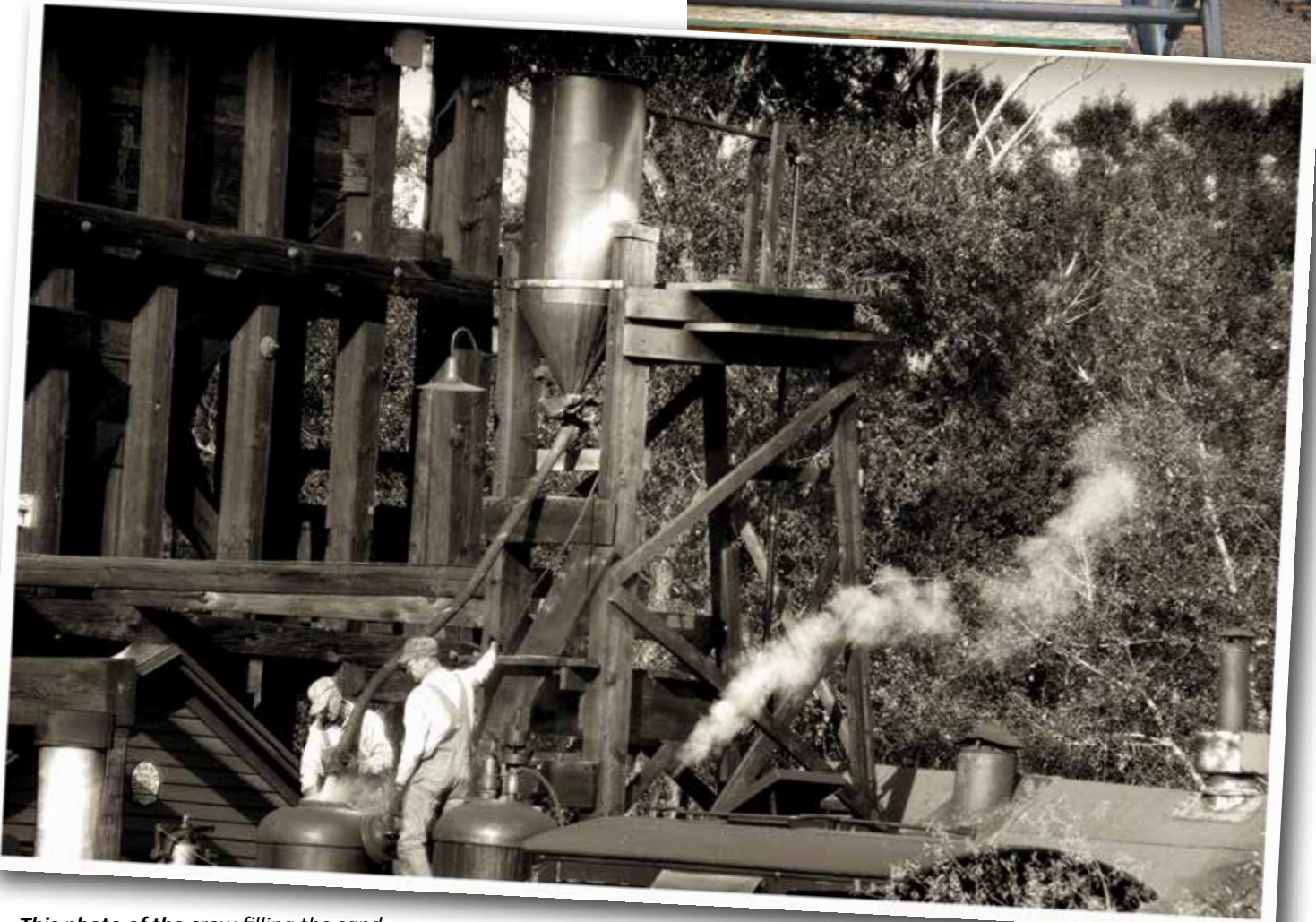
This photo of the crew filling the sand dome of D&RG Locomotive 315 at the Chama Sand Tower in August, 2017, could just as easily have been made in August, 1927, when the Sand Tower was still new.
