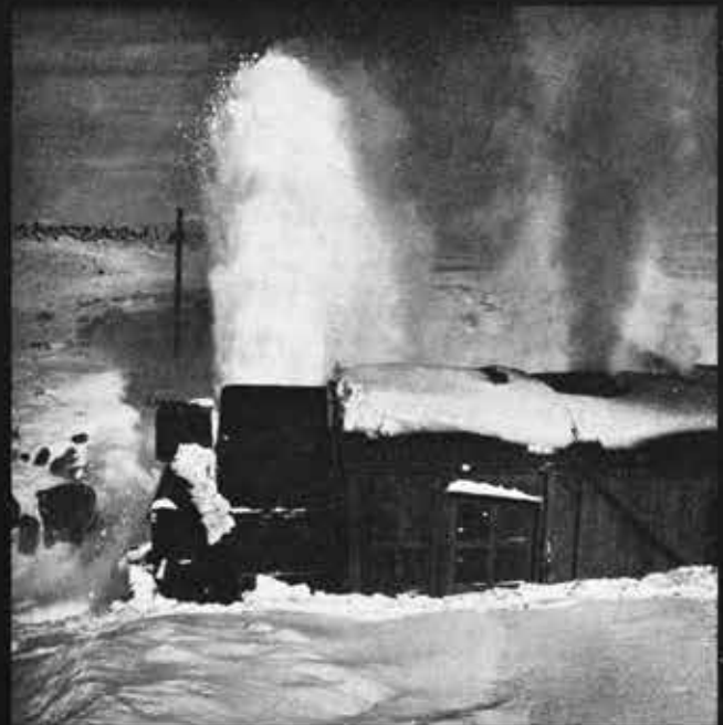
STEADFASTLY plowing ahead, steam-powered Rotary OY chews through hard-crusting snow and blasts it into the cold Colorado air. Two sweating bare-backed firemen inside heave coal into the hungry firebox as the stack erupts a steady stream of black smoke.
