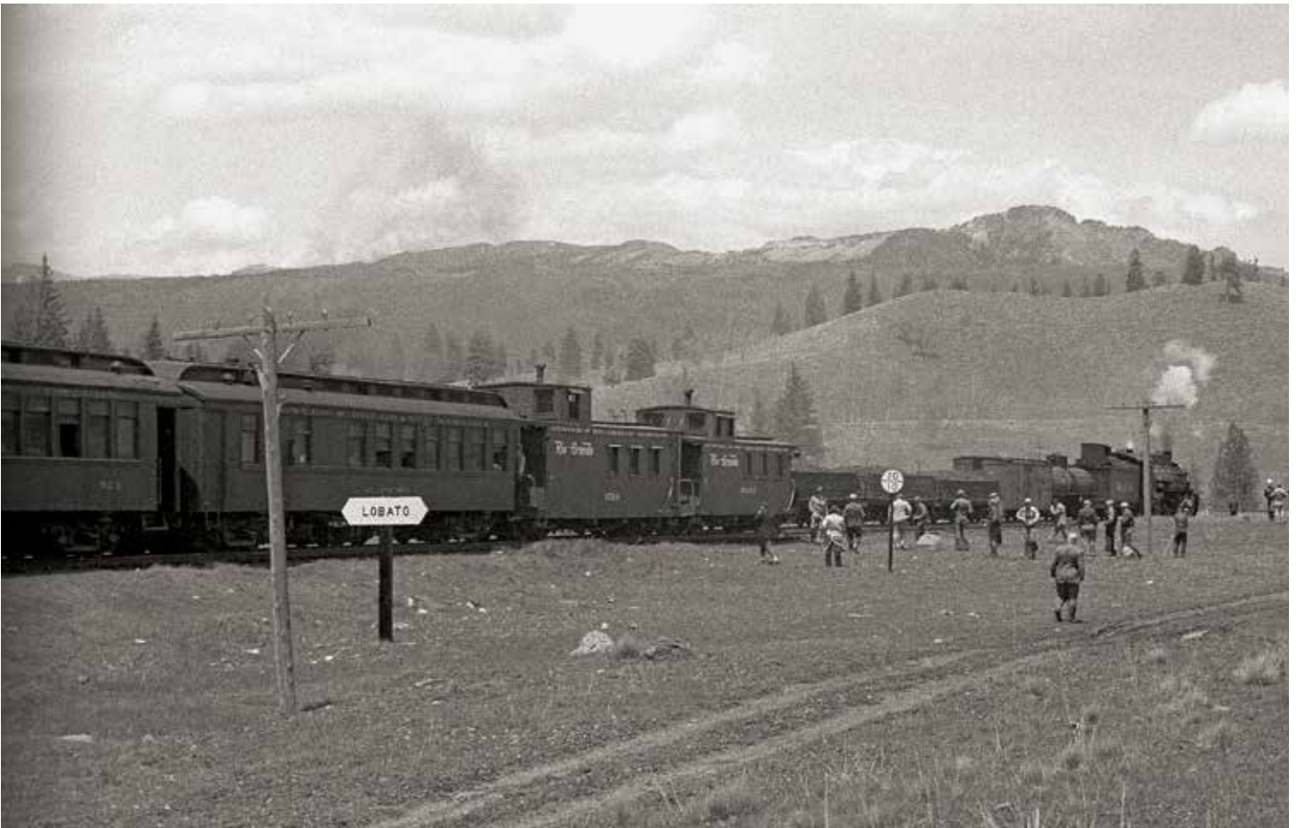
The 1954 trip in the siding at Lobato, waiting for a K-37 eastbound freight to resume its battle with gravity. The freight will quickly encounter the steep section of 4 percent grade up to Cumbres, while the RMRRC train will drift down the remaining four miles into Chama.
