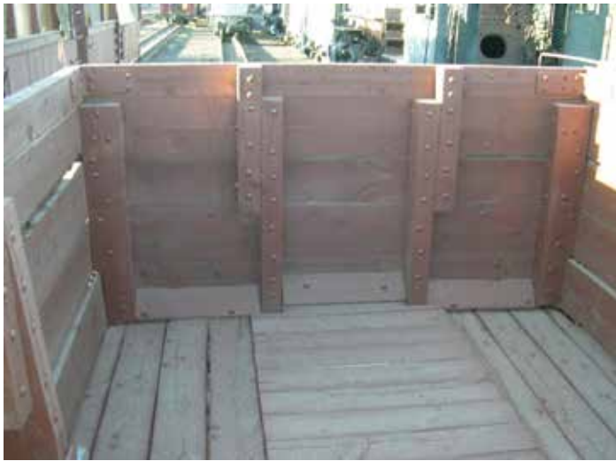
Interior view of a 800 series DBG, showing the side board extension "cripples," the corner posts used in only the 800 series cars, the drop doors on both sides and the center deck that causes a problem when unloading these cars.
