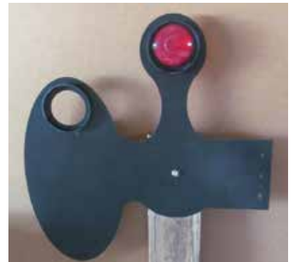
Water-jet-cut parts form a prototype for one of the semaphore arm supports. Photo by Roy Lloyd
