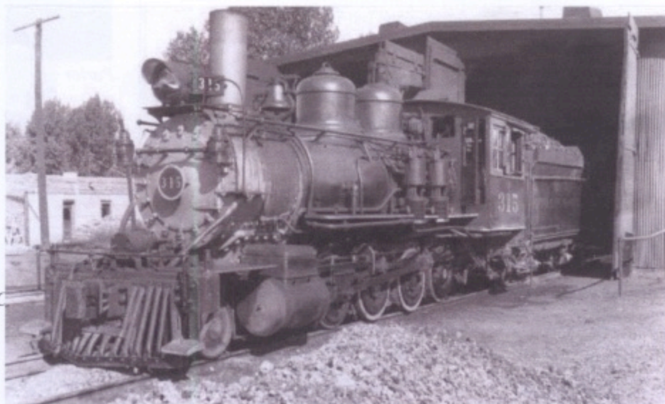
RD098-051 D&RGW engine number 315 is in road service on the Ouray branch, working out of Montrose, Colorado, on August 16, 1940, in this view by Russell F. Trepow. The air cylinder on the pilot beam raises and lowers small flanger snowplows behind (sic) the pilot wheels. Photo from the Richard L. Dorman Collection of Narrow Gauge Railroad Photographs, Friends of the Cumbres & Toltec Scenic Railroad.
