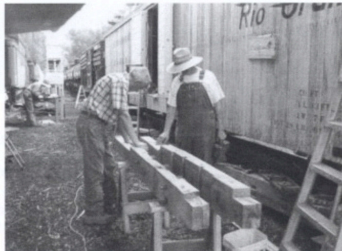
TL Bill Pratt and Randy Parks discuss cheek plate beams which secure coupler to the car.
