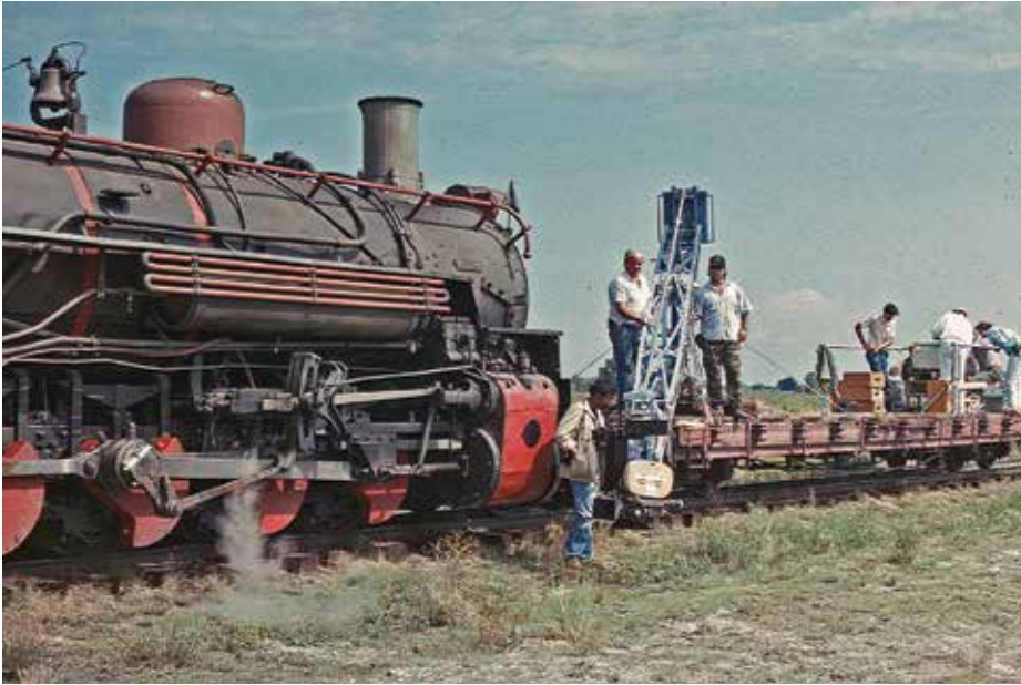
The production staff thought a movie crane on a lightweight flatcar pushed ahead of Locomotive 484 along narrow gauge track at 15 mph would be stable. It wasn't.
