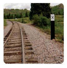
"X" lets the engineer know the train is approaching a road crossing. The engineer then blows the corresponding whistle signal until the leading locomotive is in the road.
