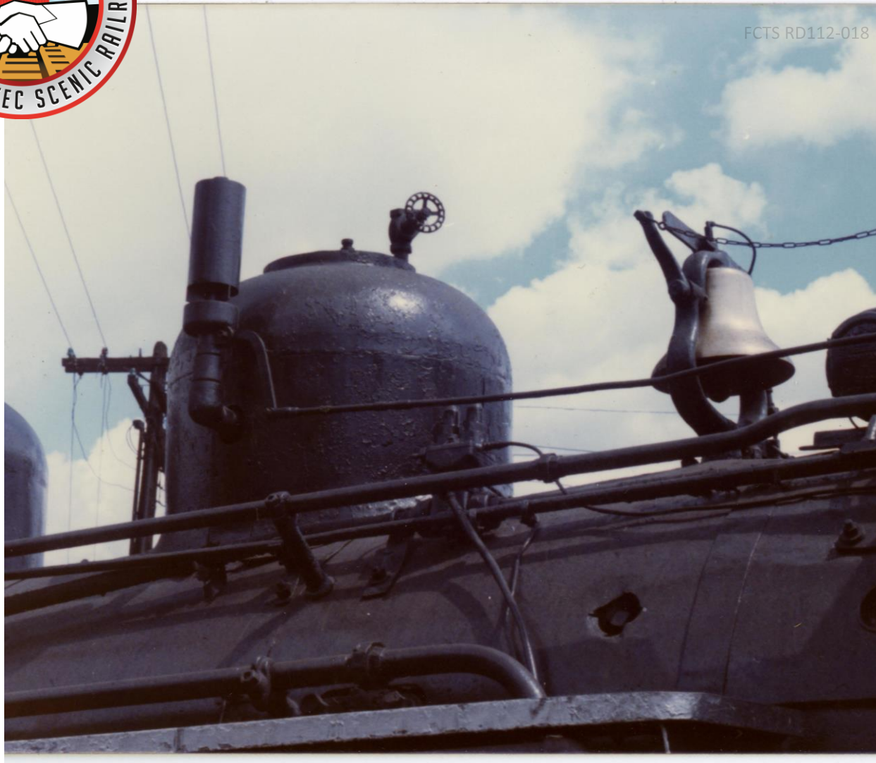
The right side of the steam dome with the whistle and bell.
