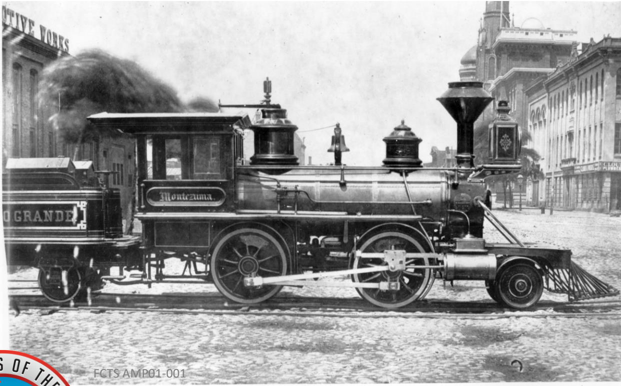
Builder's photo of D&RG #1 "Montezuma". Built in 1871 by Baldwin Locomotive Works. Notice the bell at the center. Taken circa 1871.
