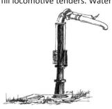
cistern on the hill above the spout. The cistern is fed by a spring several miles to the north. The cistern replaced the wooden water tank (5). The locomotives use about 3,500 gallons of water in their 14-mile climb from Chama to Cumbres.
