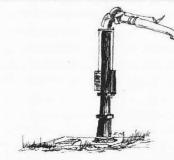
cistern on the hill above the spout. The cistern is fed by a spring several miles to the north. The cistern replaced the wooden water tank (5). The locomotives use about 3,500 gallons of water in their 14-mile climb from Chama to Cumbres.
