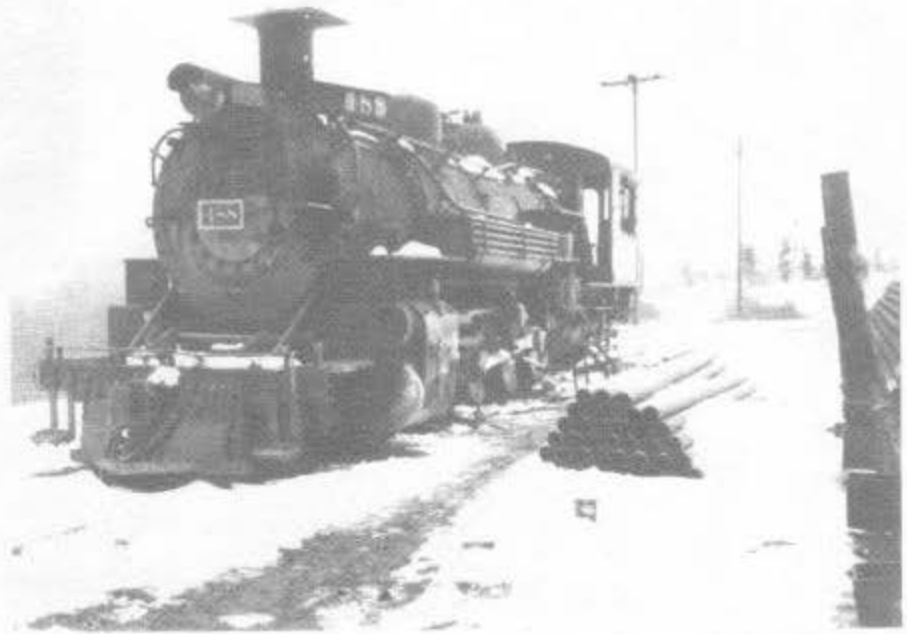
RIGHT: Locomotive No. 488 outside the Chama engine shop. Superheater boiler tubes of No. 489 are stacked on the ground.
