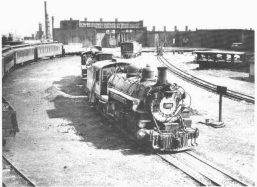
The Alamosa, CO, refinery is shown in the left background in this 1953 photograph taken by Phil Hastings in the Alamosa yard. Also in the background is the standard-gauge roundhouse, from which protrudes the tender of a 2-10-2. To the right is the narrow-gauge roundhouse. Narrow-gauge locomotives nos. 492 and 499 are moving out on the dual-gauge track. Reprinted with permission from Colorado Memories of the Narrow Gauge Circle , Carstens Publications, Inc., 1979.
