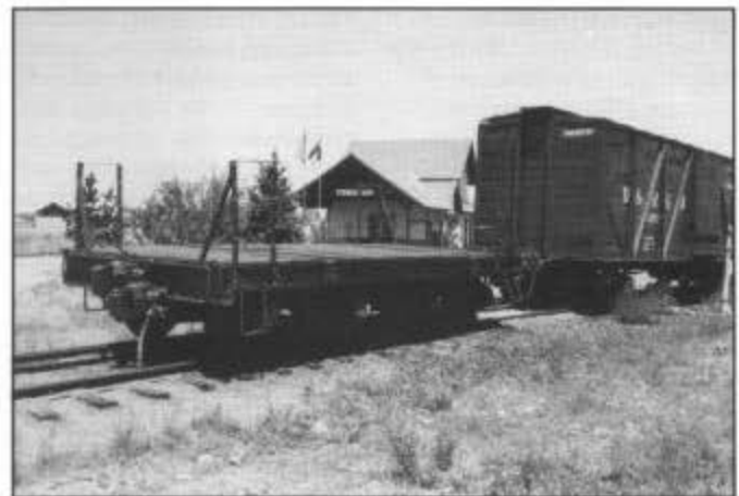
Antonito: newly painted idler car no. 010793; note both standard- and narrow-gauge couplers on the west end of the car.
