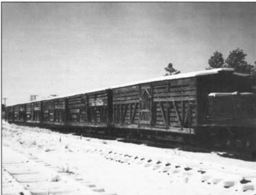
On November 23, 1992, the six stock cars are shown parked in the south end of the Chama yard. From the left, nos. 5600, 5841, 5633, 5553, 5674, and 5549. There are different side board configurations for different lettering styles. Photograph by Earl Knoob.
