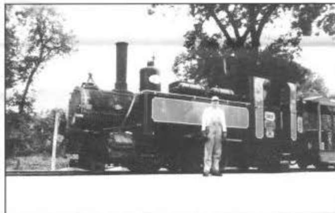
Omaha Zoo railroad's 1890 Krause 0-6-2T side tanker and engineer John E. Bush.
