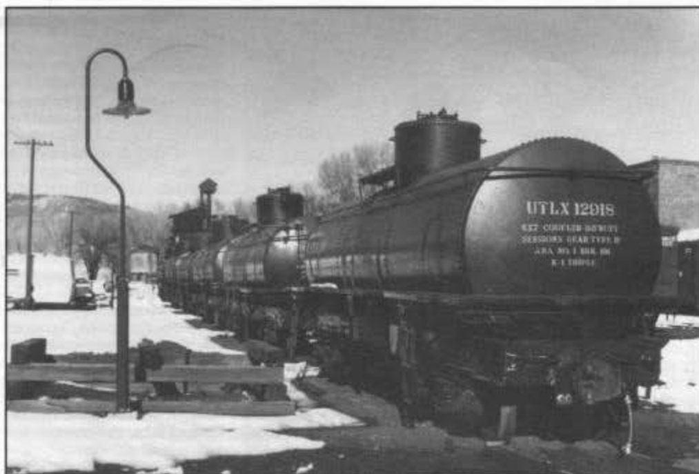
The six narrow-frame, UTLX tank cars were parked just north of the depot on January 18, 1994. Full size couplers have been installed on the cars.
