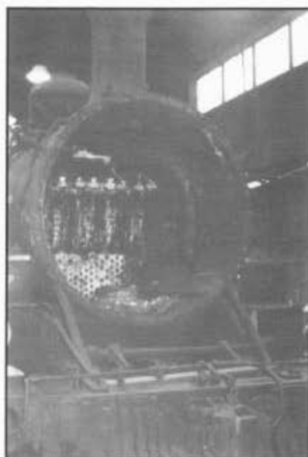
The 497's smoke box door has been removed, exposing the superheater elements.
