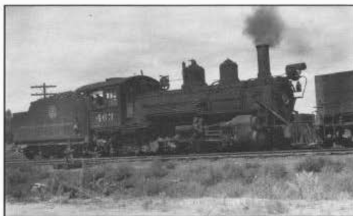
Figure 2. Still sporting a brass-rimmed number plate and six-pane windows, 463 switches the dual-gauge yard at Montrose, Colorado, on September 5, 1936. Also note the headlight without "winged" number boards. All three of these things were changed after 463 fell through the bridge at Cimarron, Colorado, on June 16, 1938. Photograph by Gerald M. Best. California State Railroad Museum.
