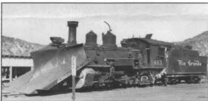
Figure 9. Engine 463 waits out the summer of 1950 next to the Durango, Colorado, roundhouse. Note the air hose on the steam dome. A length of hose was attached to this to melt ice and snow while clearing drifts from the line. August 13, 1950. Photograph by Otto Perry. Denver Public Library, Western History Department.
