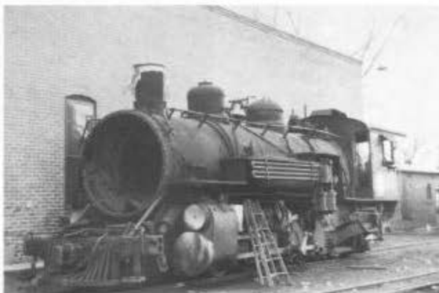
497 parked outside the old roundhouse at Chama. The engine will be reflued and the front and rear tube sheets will be replaced. May 11, 1995. Photograph by Art Nichols.
