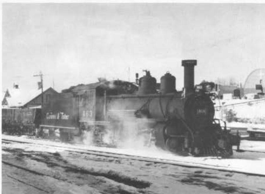
Engine 463 in the Chama yard on the morning of October 18, 1994. A deadhead move was made that day to Antonito. The consist was two gondolas of cinders, diesel 19 (towed dead), ten coaches, and caboose 0306. The helper engine was 489. Photograph by Joseph P. Hereford, Jr.
