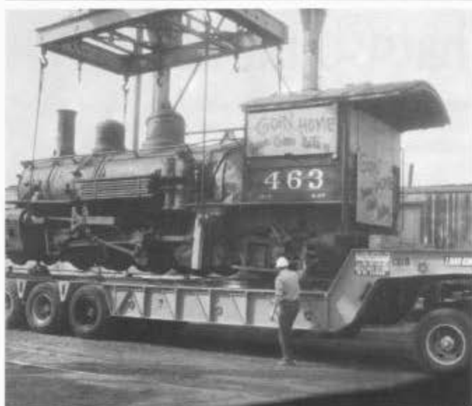
In Alamosa 463 was lowered on to a flat bed truck for the journey to Antonito. Photograph by Joe C. Johnson.
