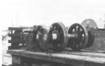
Drivers for 488 ready for unloading in the Chama yard after returning from Durango, where the tires were turned. May 11, 1995. Photograph by Art Nichols.
