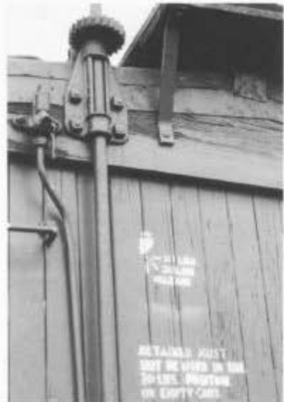
Lettering about the brake system retainer valve is on the end of the car near the brake wheel. Chama, May 11, 1995.
