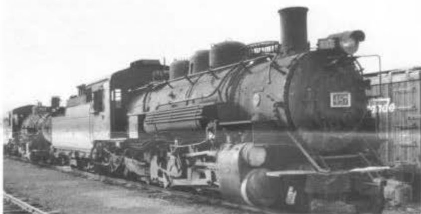
Top: Engine 484 without its plumbing, jacket, and lagging was parked just south of the Chama depot on January 11, 1996. The absence of snow was unusual for the middle of January.
