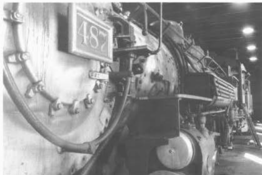
Locomotive 487's smokebox was opened in the Chama engine house, and draft appliances and the bottom two flues were removed from the boiler. 487 is under flue extension. January 17, 1997
