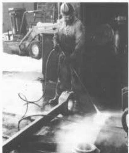
In the Chama engine house, Tommy Garcia uses a high-pressure cleaner on rods in preparation for bearing inspection. February 11, 1997
