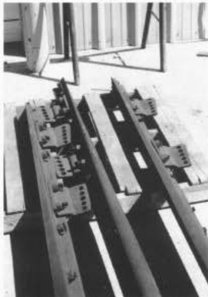
Right-hand switch points ready for cleaning.
