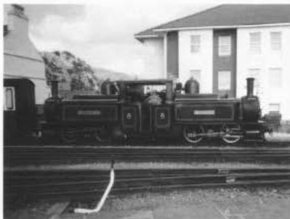
A Fairlie's double-boiler patent locomotive at Porthmadog Harbour Station on the Ffestiniog Railway. This type of locomotive was first used on the railway in 1869. Photos by Guy Combe.
