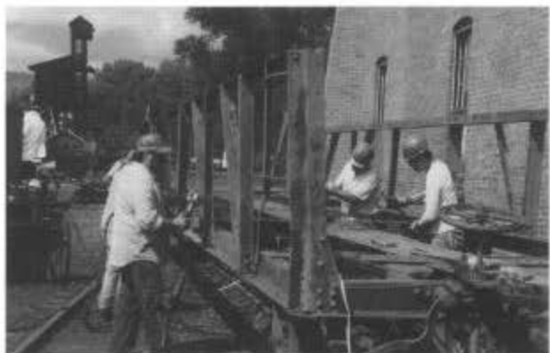
A mini work session was held in Chama the week before the regular August work session. Here volunteers remove rust from pipe gondola 9613, which was restored to be used as an observation gondola.
