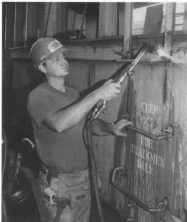
In Chama, Roy Blizzard uses an acetylene torch to cut off old bolts on a boxcar coach. All grab irons were reattached with new bolts and washers to make them more secure.
