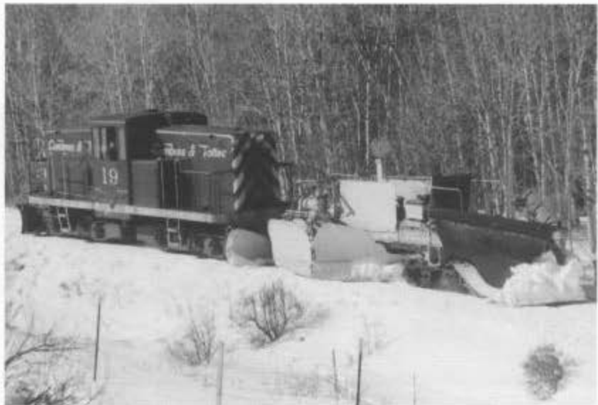
C&TS diesel 19 pushing flanger OL with plow fitted on front. Plow is from a highway snowplow. December 15, 1997 at milepost 342.
