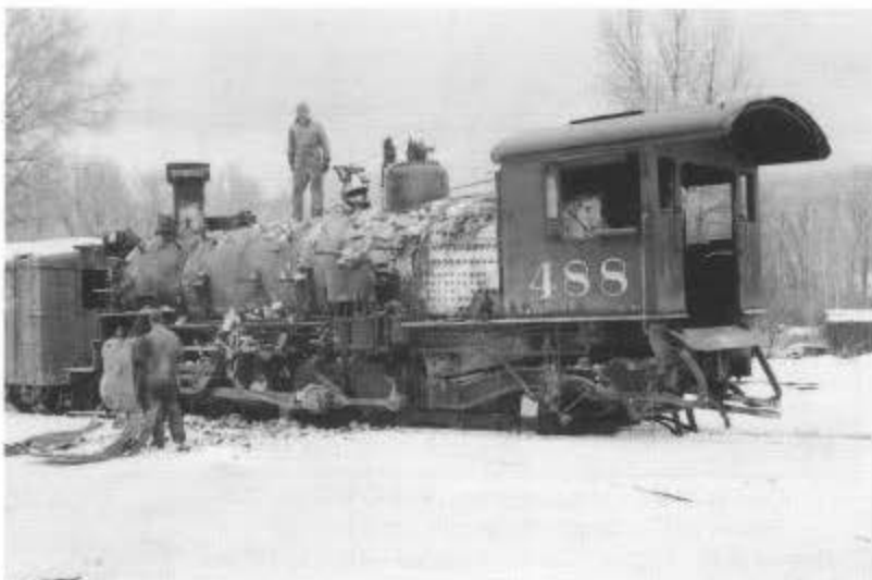
Engine house crew removes lagging from 488 in the Chama yard, November 14, 1997.
