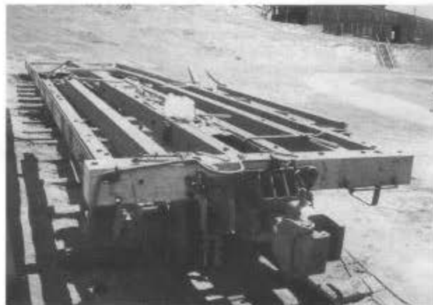
6200 with the new longitudinal and end sills in place, April 4, 1998. Bob Tully photo.
