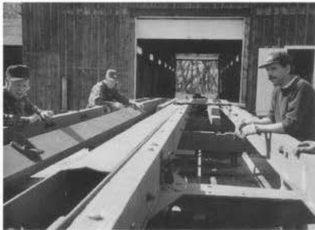
Limon Niblack (L), George Knauff, and Mike Smith inspect the new longitudinal sills, fabricated by splicing 18-foot beams (such splicing was commonly done by the Rio Grande). Roger Briggs photo.
