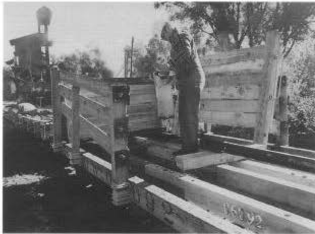
Ken Earle sprays linseed oil on all new and old sills on wheel and tie car 06092, August 1998. The new end bulkheads that will be installed next year are leaning against the side posts. In the lower right-hand corner, the identification number of the car can be seen on the new piece of the intermediate sill. Volunteers attached such metal numbers to the rolling stock collection in 1995 and 1996.
