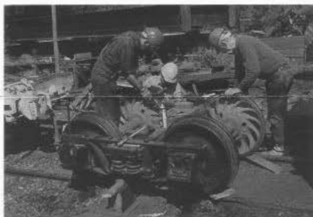
Scott Hardy (left), Art Randall, and Clint Collins change a journal box on a truck from stock car 5633, August 1998.
