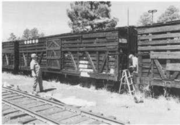
Dick Caldwell eyeballs the alignment and spacing of stencils prior to lettering stock car 5549, with 1926-style lettering, at Chama, June 1998. (Terry Woolsey)
