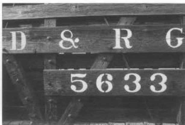
Top: Seven-inch lettering done with a paint sprayer showing overspray. Bottom: Crisp edges on 7-inch letters done with stencil brush, Chama, January 1999. (Tom Cardin)
