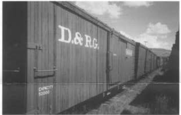
The lettering crew applied 1892-style lettering to boxcar 04444, one of the oldest unmodified freight cars in service on the C&TS. The crew lettered seven cars during sessions A and B. (George Swain)
