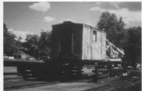
The superstructure on cribbing with the flat car removed, before being lowered onto a flatbed truck for the trip to Colorado Springs. (Ken Spencer)
