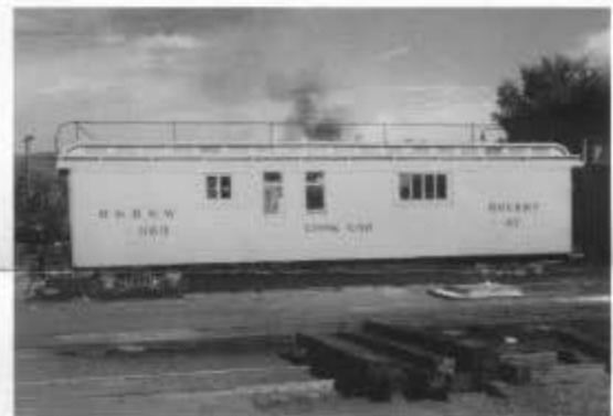
Railway Post Office (RPO)/Cook Car 053 in the Chama yard at the end of the June work sessions. Volunteers completed the end platform work begun in 1997 by installing new steps. They also relettered the car. 053 was built as a 30-foot RPO in 1885 and served for many years on the Chili line between Santa Fe, New Mexico, and Alamosa, Colorado.
