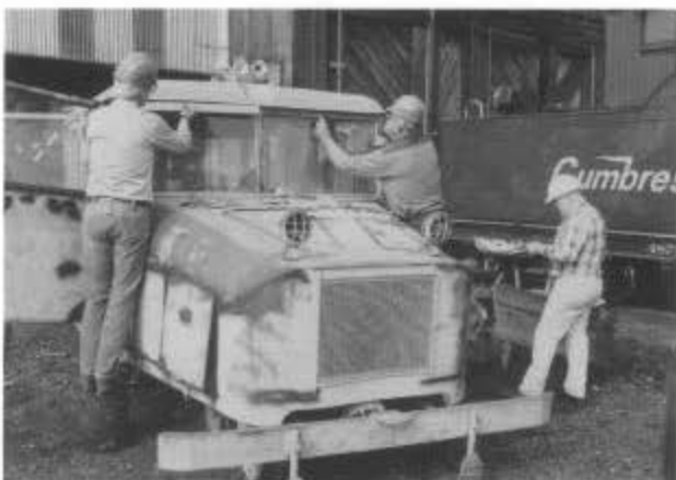
In front of the old roundhouse in Chama during session A, Gus Wurtzer and crew replace a window frame on inspection car MW02. Work on this car will continue in 2000.
