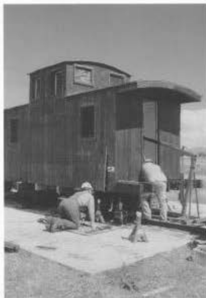
Short caboose 0579 on the repair-in-place (RIP) track in the Antonito yard. On each side of the track are the 8- by 160-foot concrete aprons the Friends installed in 1997, which provide a suitable surface for working under cars (session D).
