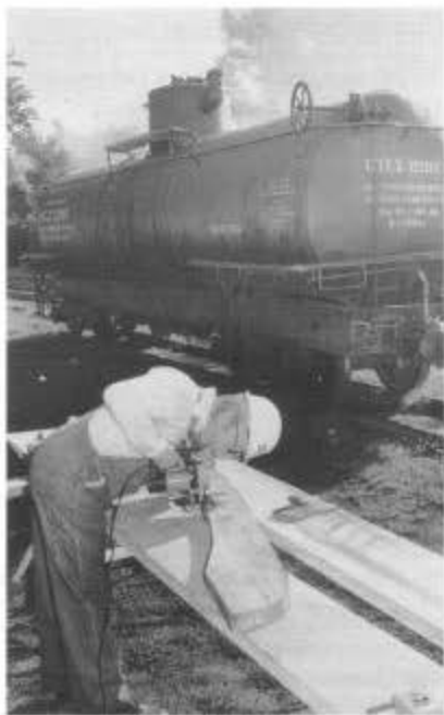
In the Chama yard during session C, Ken Earle saws a notch in the end walkway for tank car 12918.
