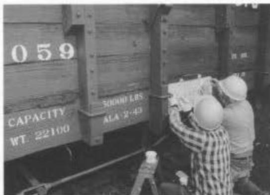
Bob Gotthelf and Edward Seidel stencil flat-bottom gondola 1059 in the Chama yard (session C).
