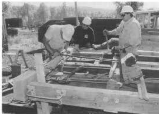
In the Chama yard during session C, Roy Blizzard (left) and Dave Sands guide the end sill on to wheel and tie car 06092 while Tony Kassin uses a come-along to draw it into position.
