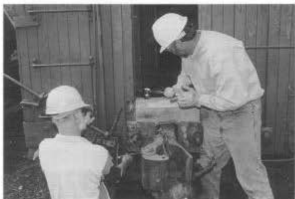
Andy Ross (left) and Ron Ross tighten bolts on the coupler pocket of water service car 04904 in the Chama yard during session C.
