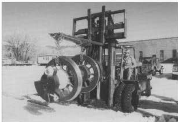
Gerald Blea unloads newly turned drivers for 497. The flange profiles were turned in Durango. (Photos by Tom Cardin.)
