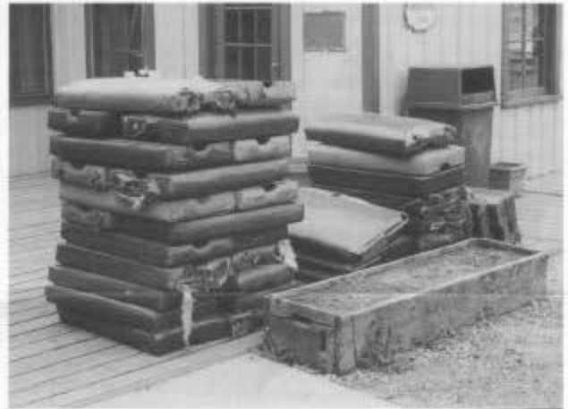
Outside the Chama depot, torn seats and seat backs from the coaches are ready to be sent for re-covering.
