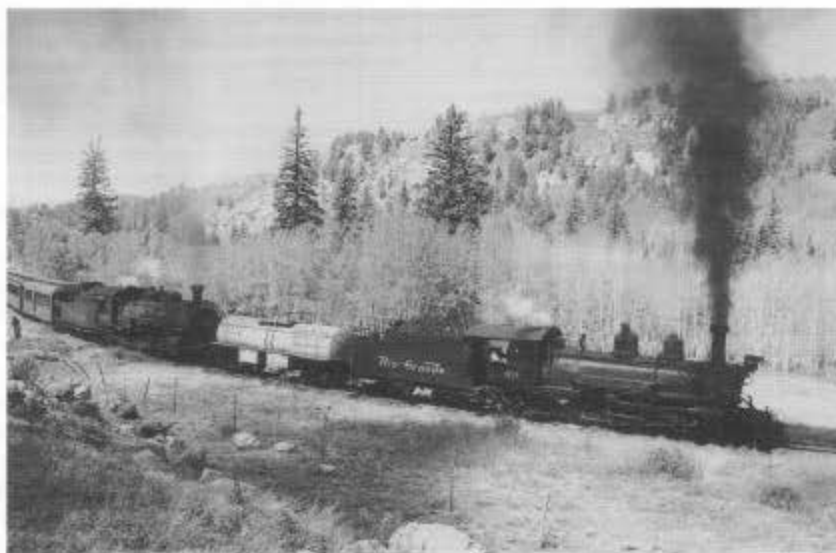
The eastbound train from Chama on Saturday, May 27, 2000, coming out of the Narrows. Locomotive 463 is the helper and 489 the road engine. To reduce the risk of fires, Rotary Snowplow OY's water car sprayed water along the right of way. (Photo by Tom Cardin.)
