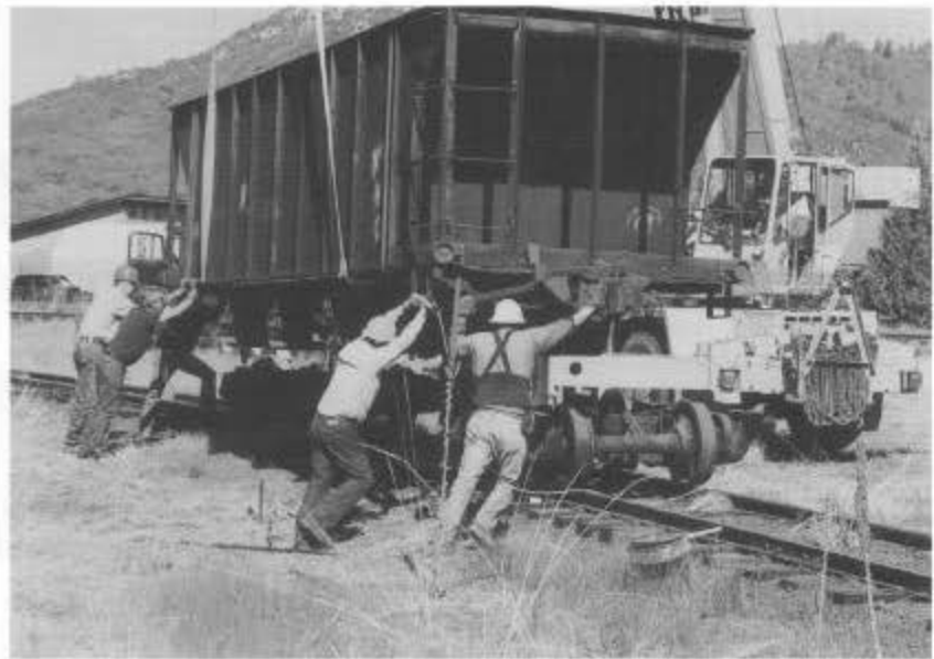
Lowering one of the ex-East Broad Top hoppers onto its trucks at the wye in Chama. The Cumbres & Toltec Scenic Railroad Commission purchased five of these hoppers from the East Broad Top, two of which were brought to Chama on flatbed trucks during the May volunteer work sessions. The commission purchased the cars with funds from the Economic Development Administration grant for track rehabilitation. The cars will provide an efficient way to move ballast; the historic fleet doesn't include any hoppers. The drop-bottom gondolas in the historic fleet are not robust enough for rigorous regular service, and they dump along the outside of the rails, requiring manual shoveling. (Photo by Tom Cardin.)
