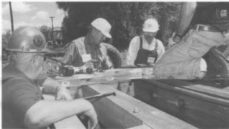
Geof Gordon tightens a truss-rod on flat car 6214, while Jim Phelps (left), William Hurry, and Mike Wissler stand by to assist (session A). Below, members of the passenger car team work on the interior of coach 524, Los Pinos. They repaired paneling, trim, flooring, and seats (session B). (Photo by George Swain.)
