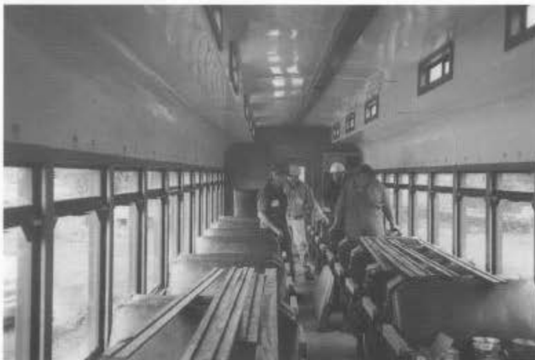
Geof Gordon tightens a truss-rod on flat car 6214, while Jim Phelps (left), William Hurry, and Mike Wissler stand by to assist (session A). Below, members of the passenger car team work on the interior of coach 524, Los Pinos. They repaired paneling, trim, flooring, and seats (session B). (Photo by George Swain.)
