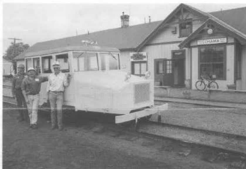
Restoration of inspection car MW02 was completed during the June work sessions. Here, Gus Wurtzer (left), Don Huber, and Joe Phelps stand beside MW02 parked in front of the Chama depot on June 30, 2000. Originally built by Fairmont, probably in the 1930s, it is powered by a Ford V-8 of about 1947 vintage. Restoration began in 1996. (All photos by Tom Cardin except where noted.)
