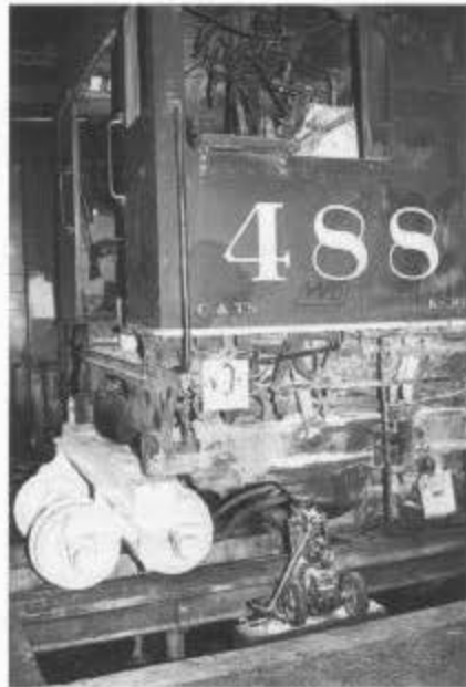
The new narrow-gauge shop trucks fabricated from standard-gauge ones. The shop trucks allow the engine to be moved while the lead and trailing trucks are being refurbished. (March 2001.)
