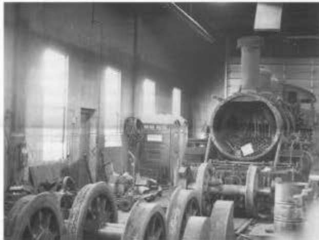
Engine 463 in the Chama enginehouse. The drivers have been removed and the smoke box door has been removed for access to the flues. (February 2001.)
