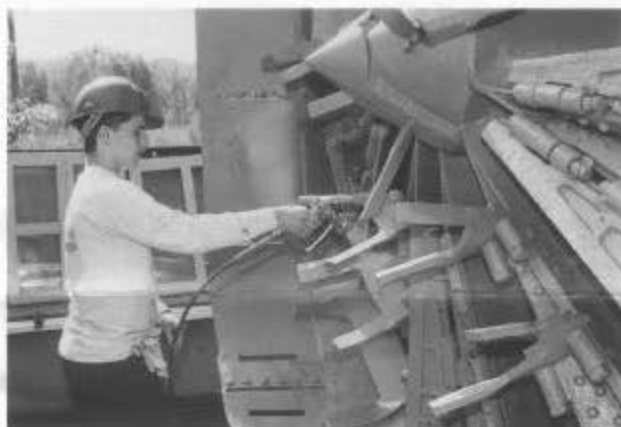
Levi Craig sprays a coat of gray on the blades of rotary snowplow OY (Chama, session B).
