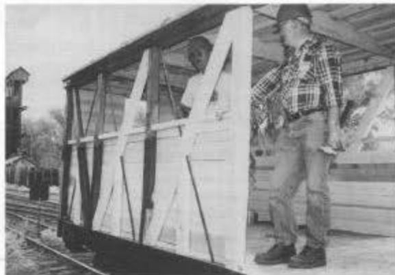
In the Chama yard, Tim Bristow (l) and George Detwiler replace the interior siding of boxcar 3605 during work session B. At right, in Antonito during session B, from the left, Warren Ringer, Jim Laycock, Jack Salisbury, Norman Grant, and Keith Hayes install a coupler on idler flat car 6708. Art Randall works under the car. (Photo by Art Nichols.)
