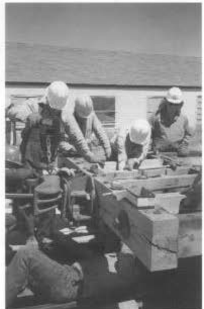
In the Chama yard, Tim Bristow (l) and George Detwiler replace the interior siding of boxcar 3605 during work session B. At right, in Antonito during session B, from the left, Warren Ringer, Jim Laycock, Jack Salisbury, Norman Grant, and Keith Hayes install a coupler on idler flat car 6708. Art Randall works under the car. (Photo by Art Nichols.)
