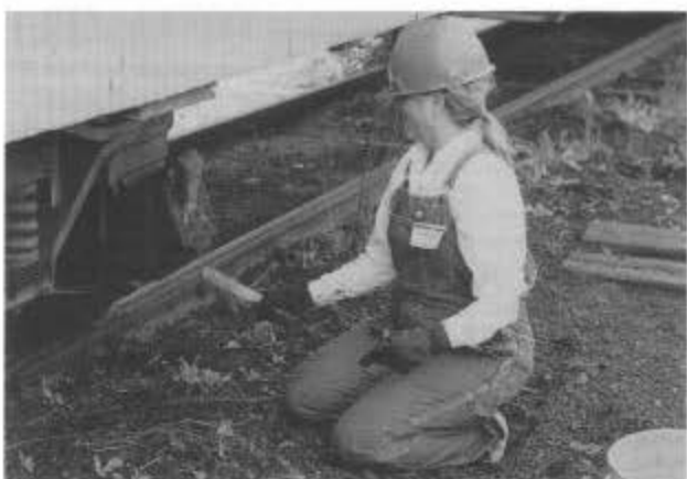
Caroline Tower wire brushes the under carriage of cook car 053 in preparation for painting. Chama, session C. (Photo by Tom Cardin.)
