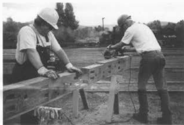
John Manion (l) and Richard McLean prepare an oak end sill for boxcar 3339 in the Chama yard, session D. (Photo by Terri Shaw.) Below, Walt Sommer (l) and Dick Seelye work on the table saw while Ron Schnitt uses the miter box and saw in the Cumbres section house during session C. (Photo by Tom Cardin.)
