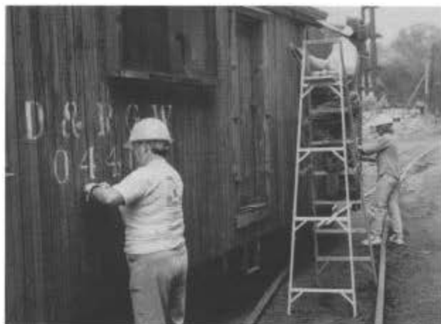
Sharon McGee (l), Tom Casper, and Joyce Rumschlag use scrapers to remove old paint from the section men's car in the Chama yard during work session D. (Photo by Tom Cardin.)
