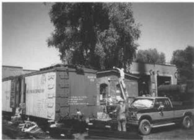
Volunteers painting the oil house. The short reefer, car 55, jacked up and placed on cribbing to take out the warp in the whole car. Chama, session C. (Photo by George Swain.)
