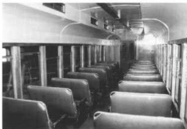
Interior of a newly refurbished coach. Seat and mechanisms have been checked and repaired where needed, and new floors laid using individual tiles so they may be replaced as needed, without laying an entire floor (Antonito, February 2002).
