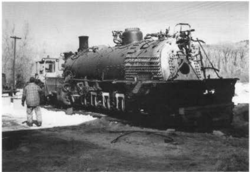
Ricky Rivas guides the loader as it pushes locomotive 484 back into the Chama enginehouse on February 20, 2002. The engine was moved outside earlier in February so that the cab could be removed, allowing access to the staybolts. The narrow-gauge shop trucks help support the locomotive; only the lead and trailing trucks are on the rails. The drive wheels have been removed. (Photo by Tom Cardin.)
