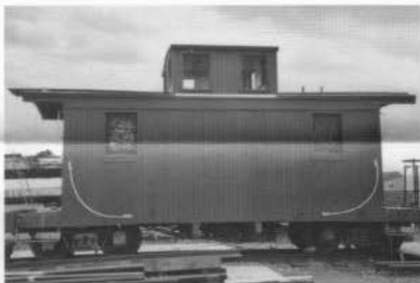
The short caboose after the session E volunteers painted the exterior and installed grab irons, hand brake gear, and the coupler on the B end of the car. (Photo by Art Nichols.)
