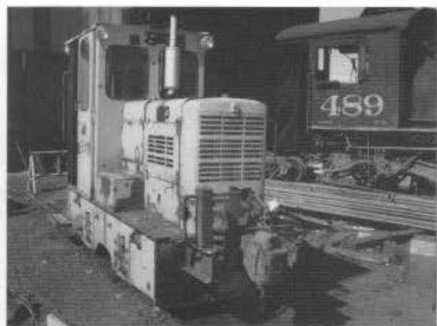
Parked outside the Chama roundhouse during session E is the 5-ton Rogers hydromotive gasoline locomotive purchased at the Sundown and Southern auction in July 2002. It will be used for switching of freight cars when a steam locomotive or the diesel 19 is not available.
