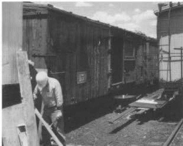
In Chama Richard Smith pulls nails from wood removed from the interior of concession car 450 (session E). In 2003 the car will be converted back to boxcar 3591. (Photo by George Swain.)
