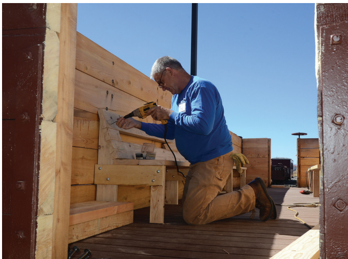
Friends of the Cumbres & Toltec volunteers upgrade a high side gondola to an open-air observation car for passengers on the C&TS.
