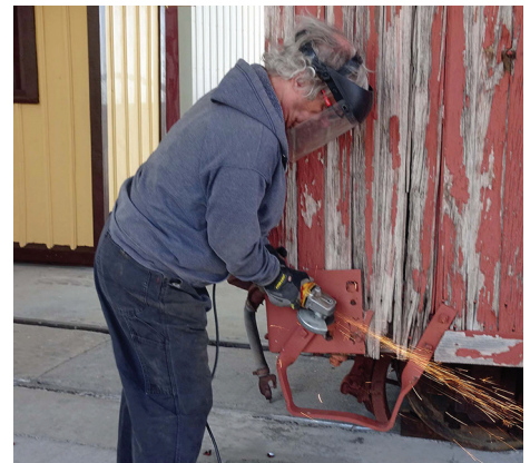
Step 3: If a wrench doesn't do the job, reach for a grinder.
